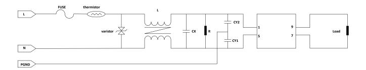
Fuse: Recommended parameters: 5A to 10A/250Vac, slow-acting fuse type Thermistor: Recommended parameters:  $2A,5\Omega,1.8W$  to 5A D10,2. $5\Omega,2.4W$ .
