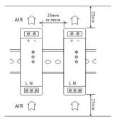
Mounting method should be considered with airflow. Leave enough space between the units when several units are mounted together. Forced air cooling makes protection against heat better.
