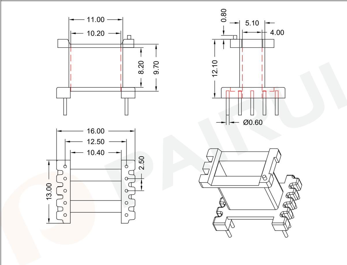
Winding data and area product for 10-pins EE/13/7/10 coil former
