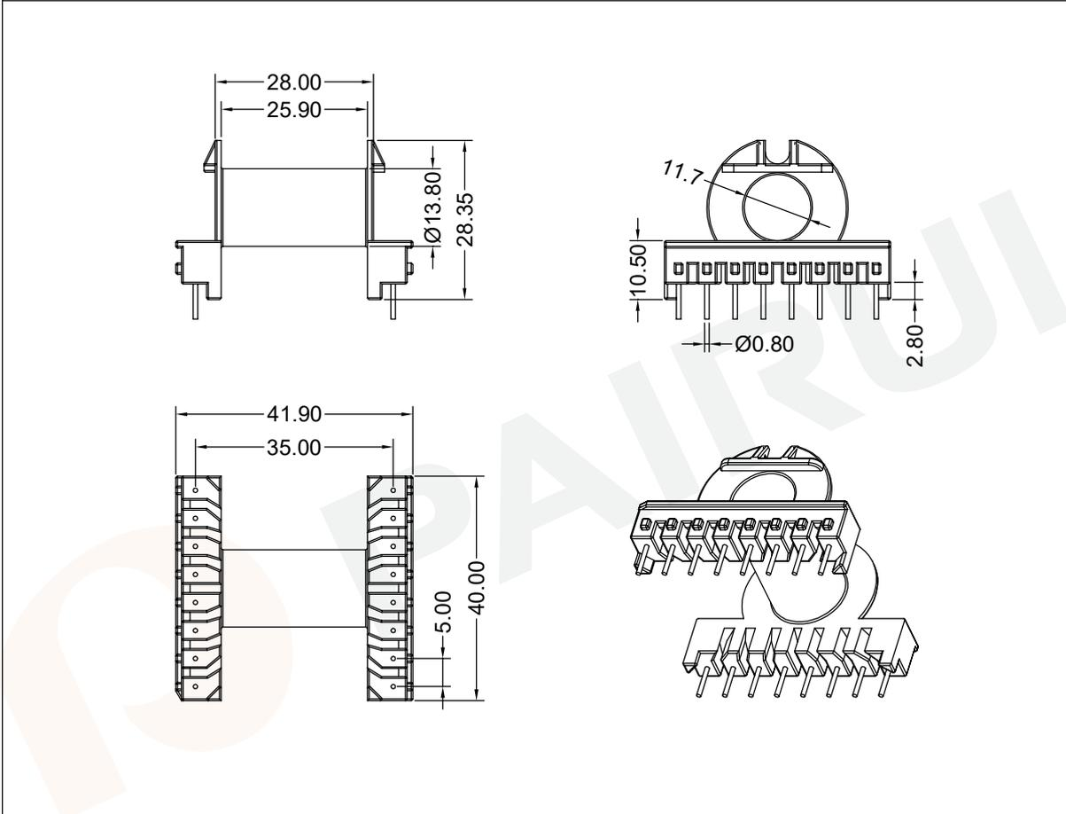
Winding data and area product for 16-pins ER35/21/11 coil former
