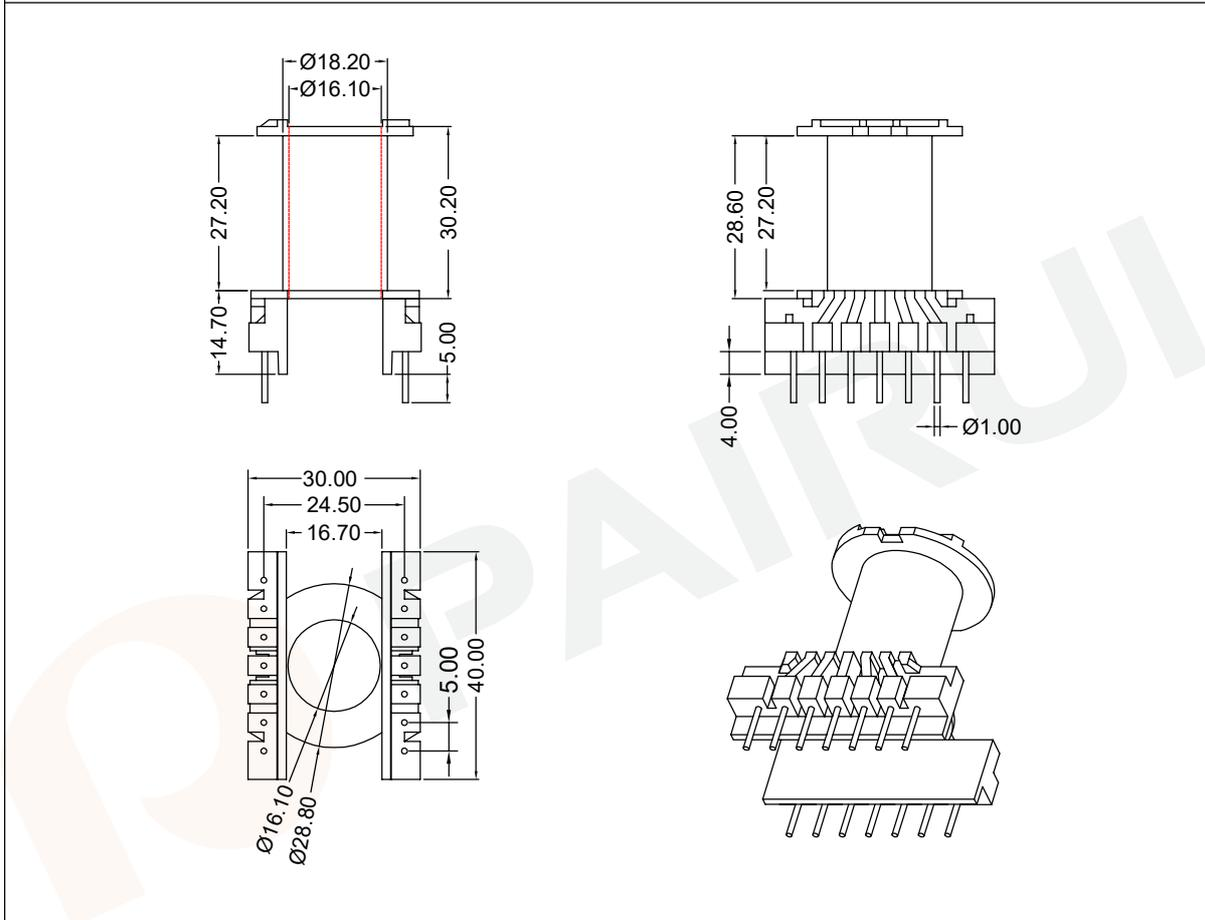
Winding data and area product for 14-pins ER42/22/15 coil former
