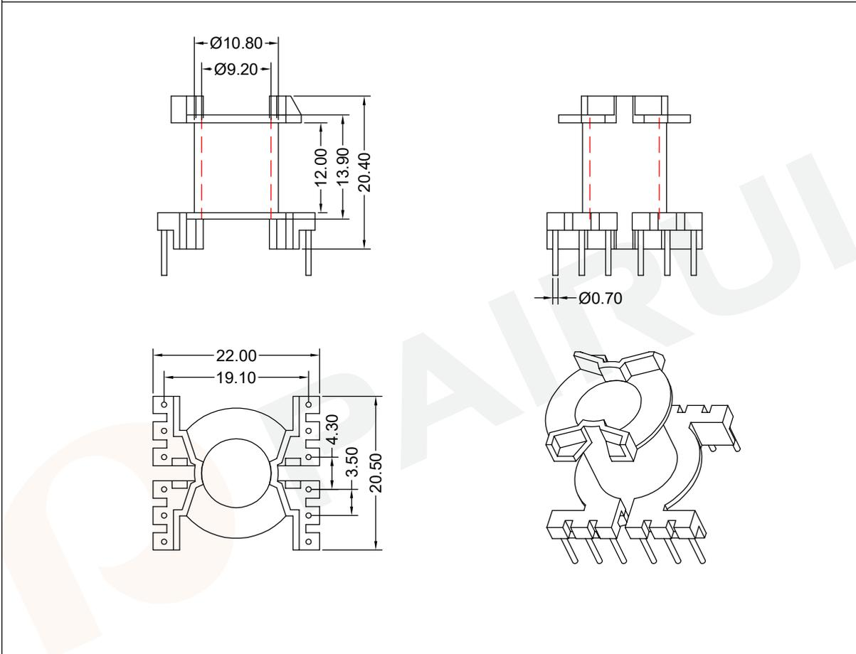
Winding data and area product for 12-pins PQ20/20 coil former
