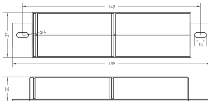
Single-layer 4-cell Lithium Battery Pack
